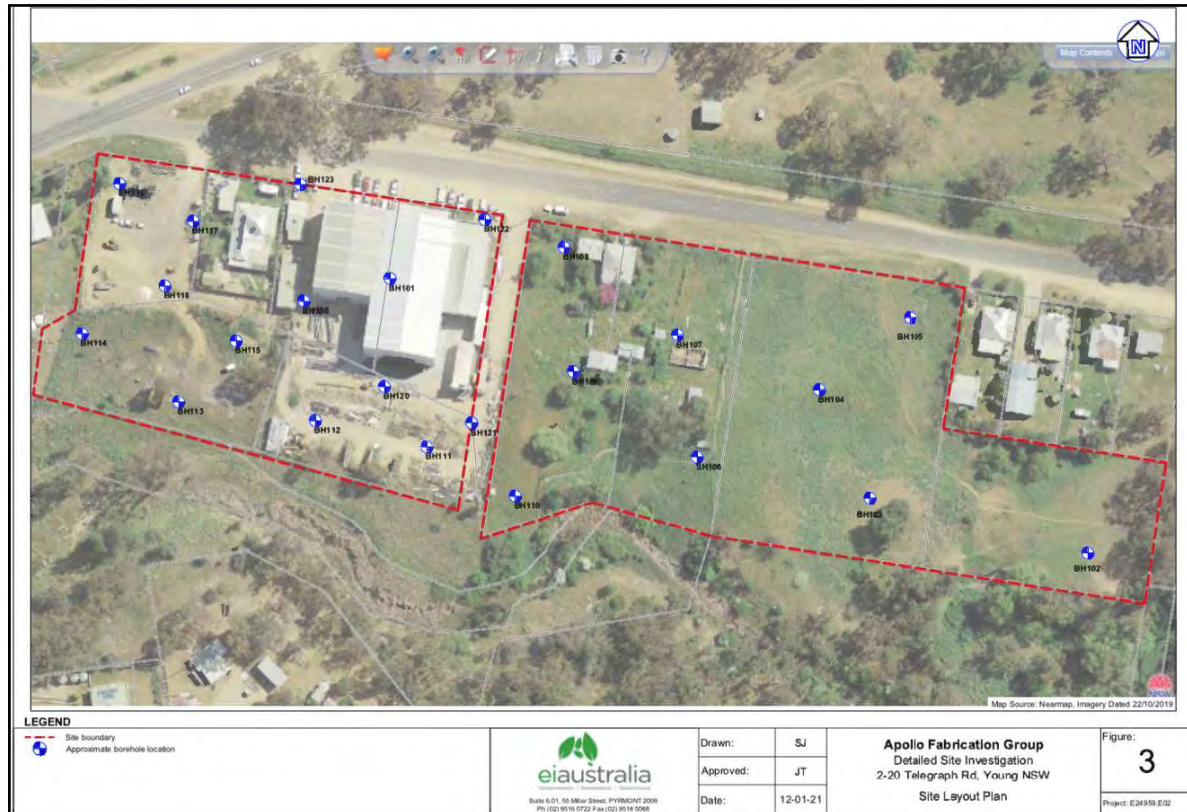
Figure 6: DSI Test Boreholes (Source: EI2021)
